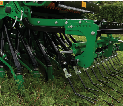
(B) Self-leveling harrow with platform and loading ladder
