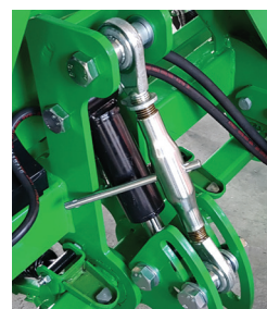
Hydraulic furrow lifting system for trailed machine
