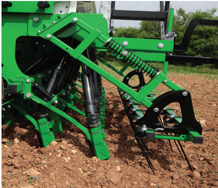
(A) Double harrow with parallelogram, with platform and loading ladder
